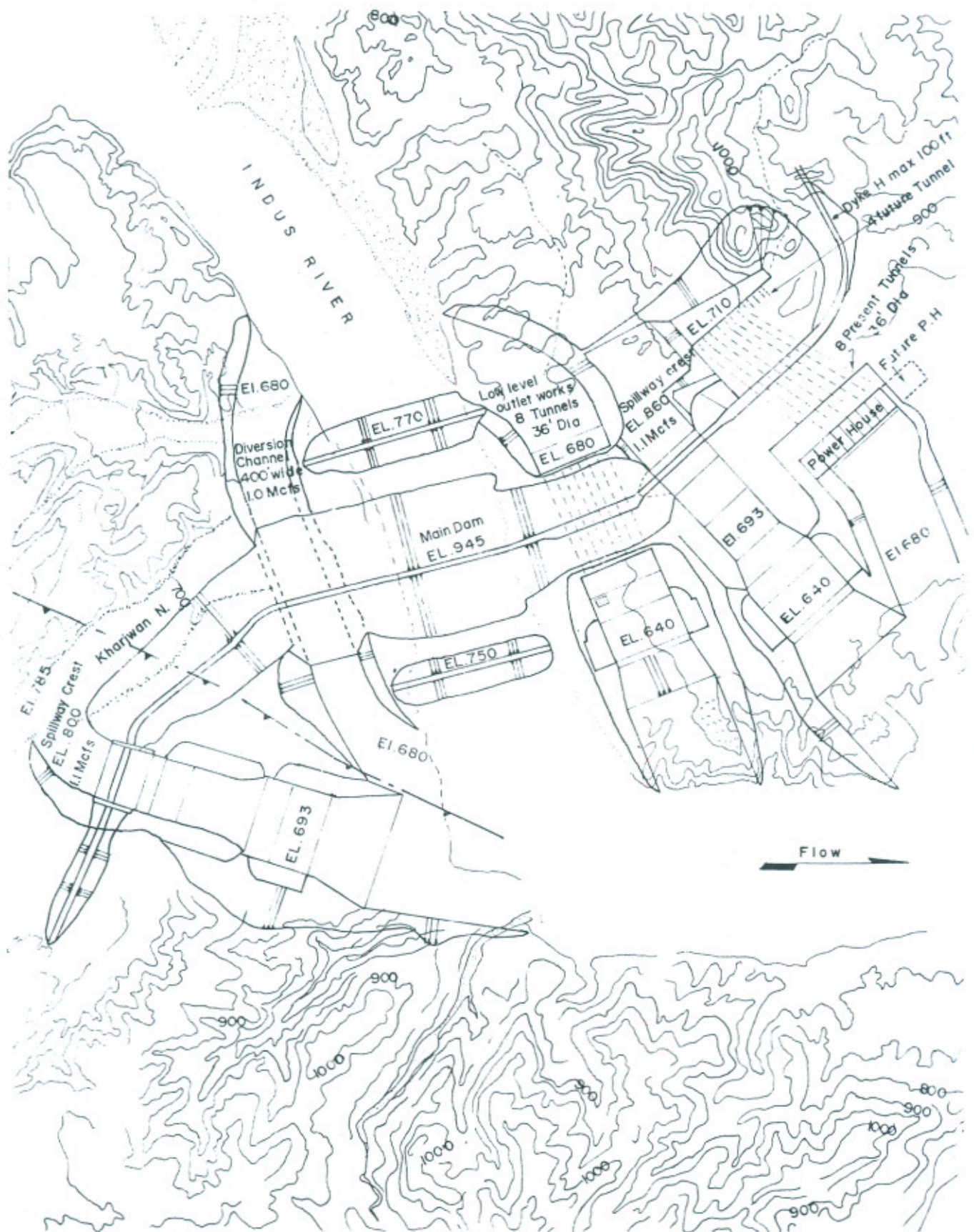
Fig.12: SITE - E LAYOUT PLAN KALABAGH DAM PROJECT
