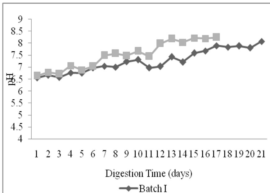
Fig. 1. Variation of pH for batch-I and batch-II
