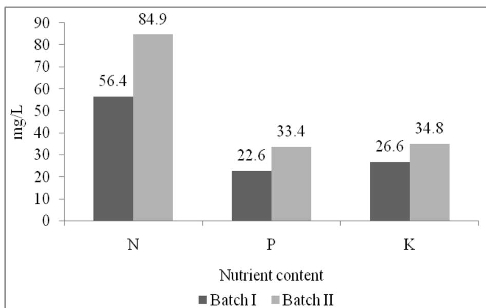
Fig. 7. NPK analysis of effluent slurry from batch-I and batch-II
