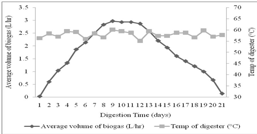
Fig. 3. Trend of biogas production for batch-I
