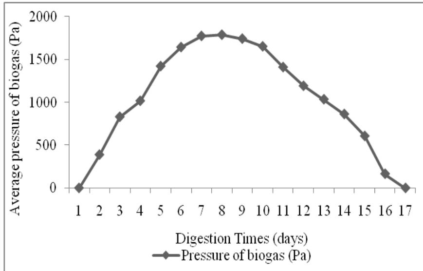
Fig. 5. Pressure of biogas for batch-II (Pa)
