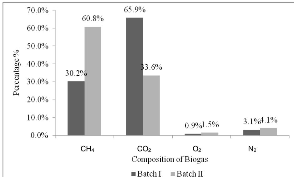
Fig. 6. Comparison of biogas composition for batch-I and batch-II
