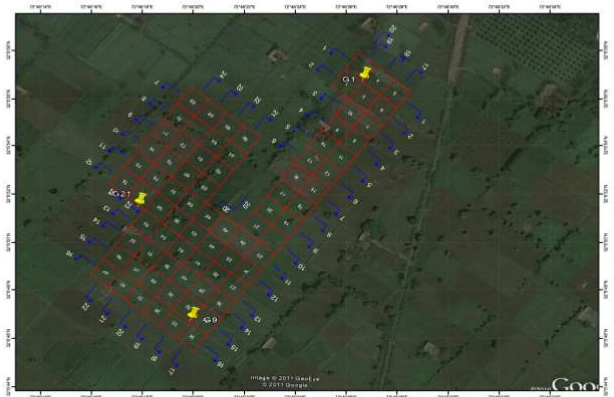
Figure 1. Geographical location of TDEM survey site - Mithalak farm (32.11297° N □ 72.77218° E) : the red squares represent the transmitting loop with its location identity and blue lines mark the geoelectric sections.
