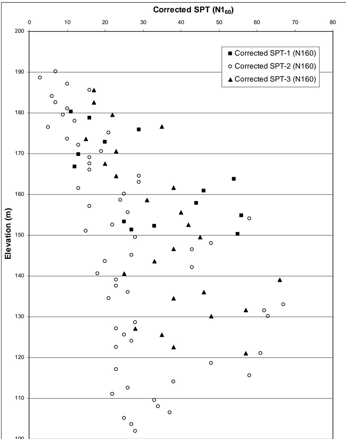
Figure 2. Variation of SPT " N CORRECTED " with elevation
