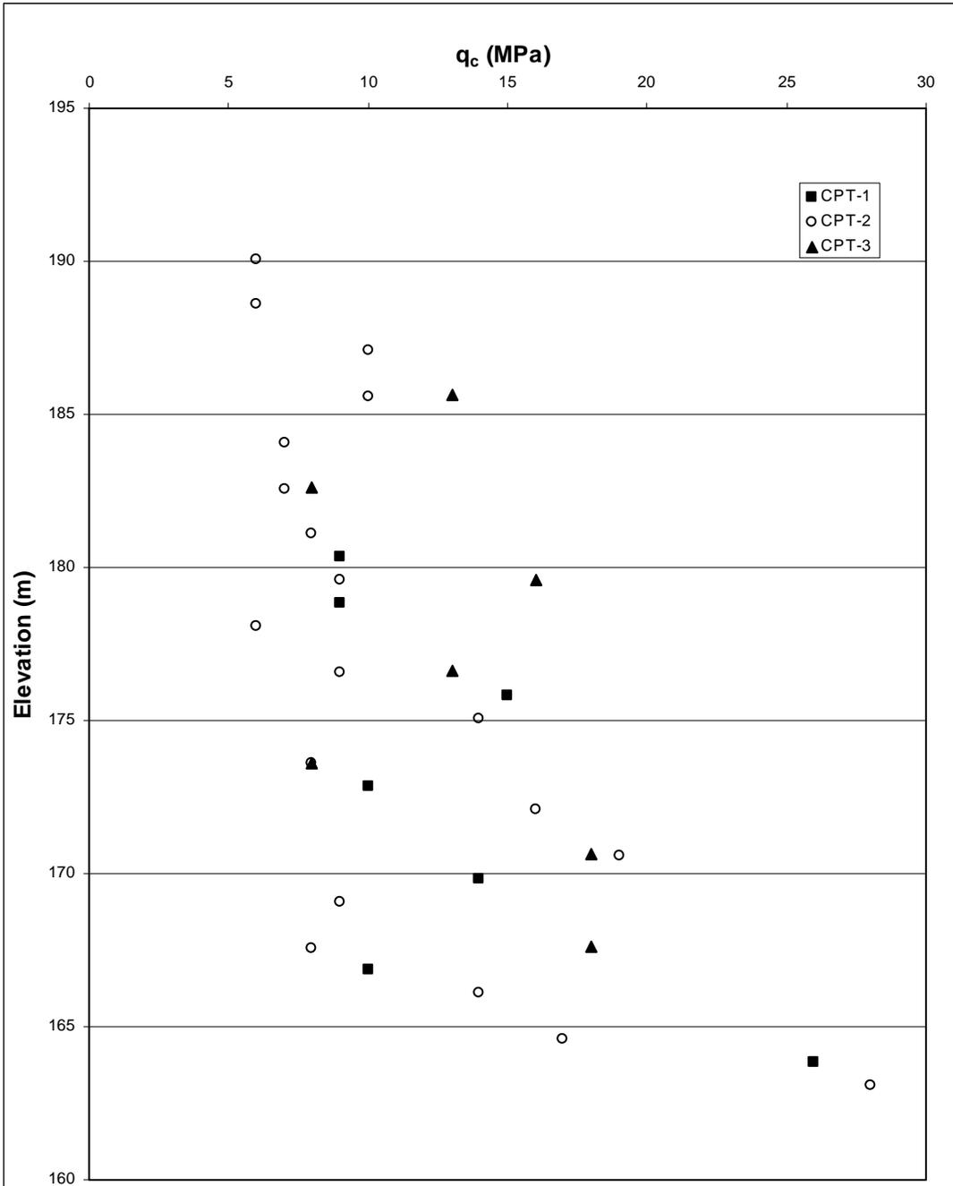
Figure 3. Variation of CPT tip resistance with elevation
