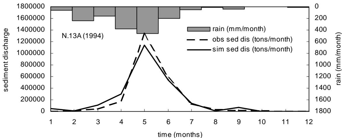
Figure 3: Simulation results of sediment discharge for Nan river basin at Ban Bun Nak (N.13A)
