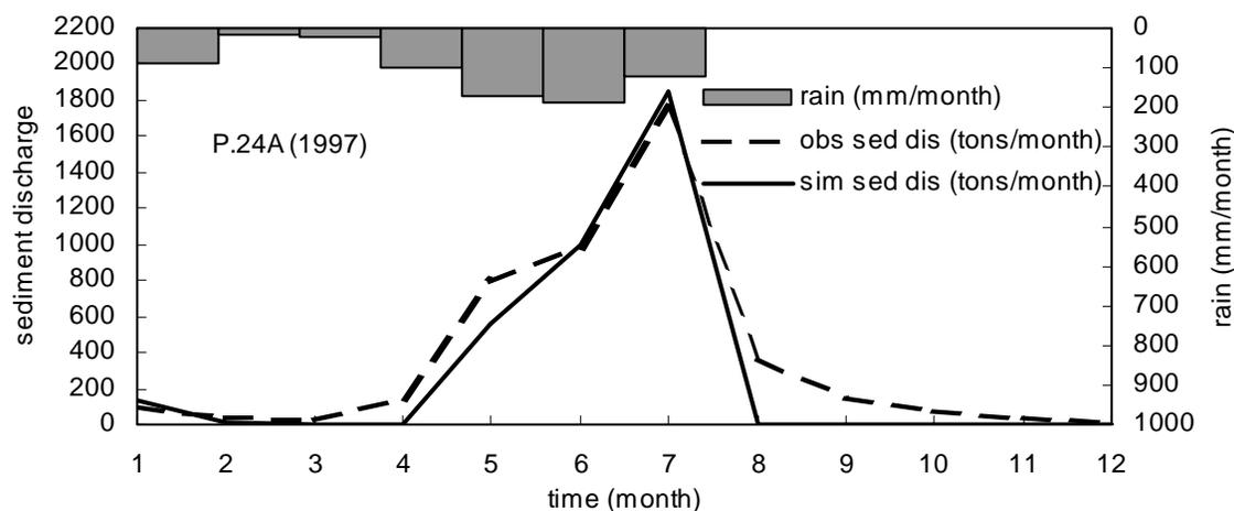
Figure 4. Simulation results of sediment discharge for Ping river basin at Nam Mae Klang (P.24A)
