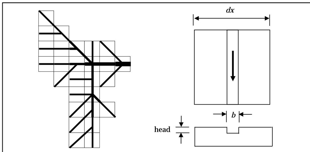
**Figure 1: Modelling soil erosion and sediment transport processes considering equivalent channel-network in the watershed.**
