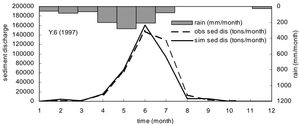
Figure 5. Simulation results of sediment discharge for Yom river basin at Ban Kaeng Luang (Y.6)
