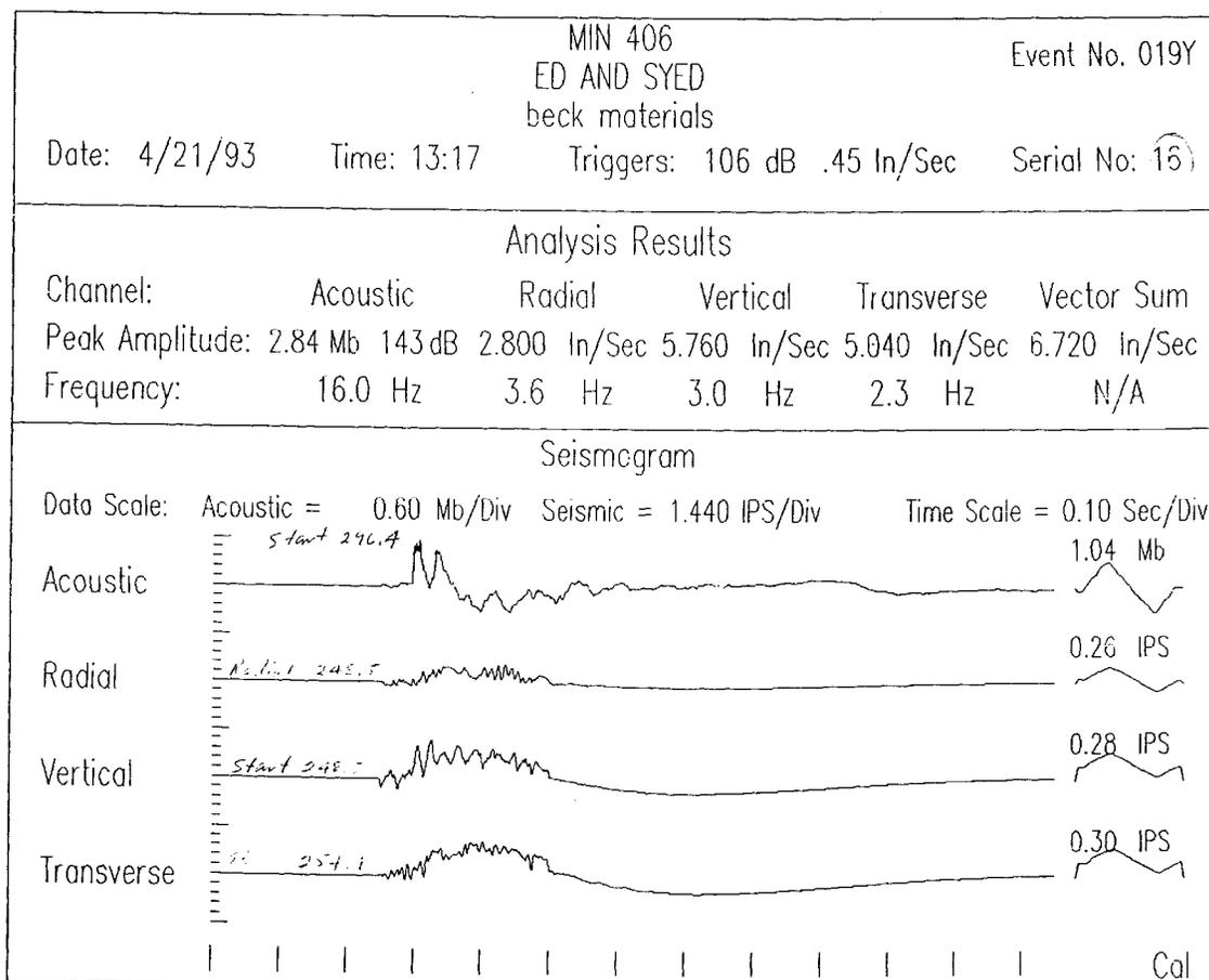
Fig. 2 A Sample Print-out of a Seismograph Reading.
