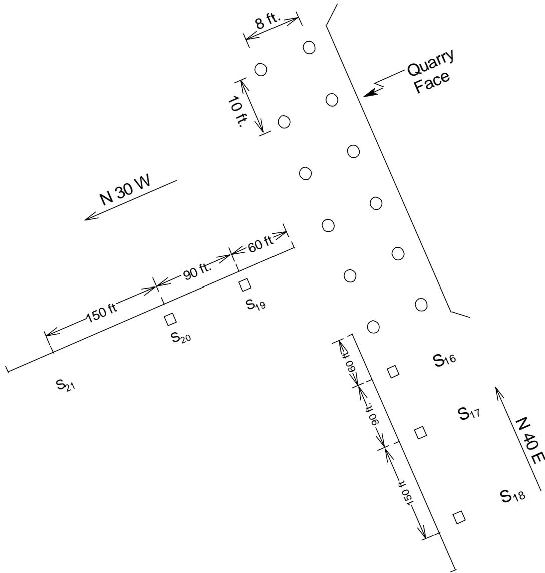
Fig. 1 Schematic Diagram Showing the Location of Seismographs in Relation to Quarry Face.
