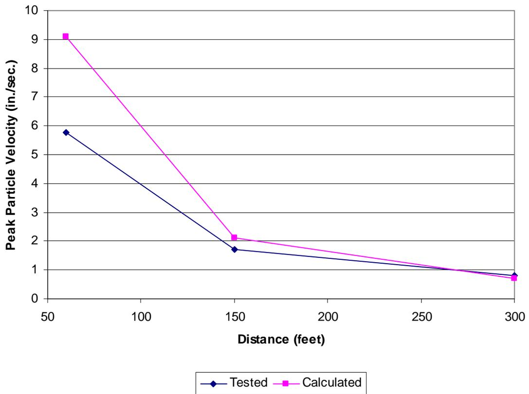
Fig. 3 Comparison of Peak Particle Velocities for Seismographs Located Parallel to Quarry Face.
