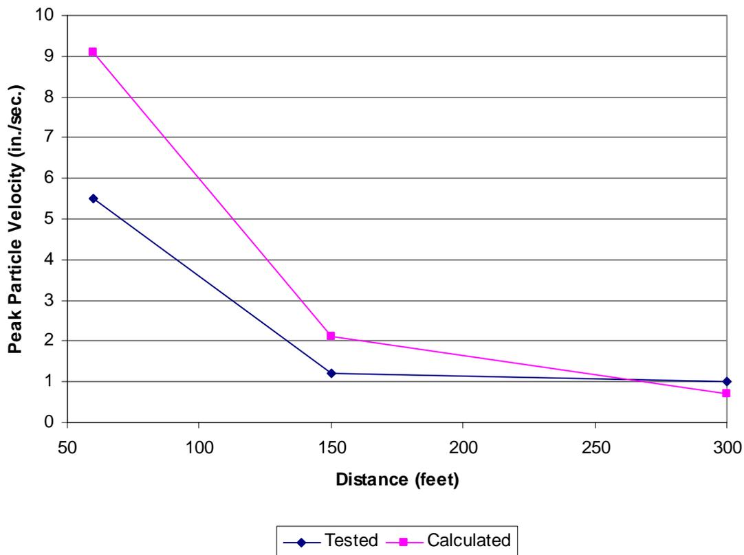
Fig. 4 Comparison of Peak Particle Velocities for Seismographs Located Perpendicular to Quarry face.
