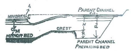
on the side of safety to limit it to 66 per cent.) For a mathematical explanation of this condition see para. XIV at the end of this note. It is necessary to limit the drowning to figure in order to make the discharge through the flume independent of the downstream supply level.
