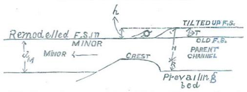
The three unknown quantities are H, h and R and to determine these we have the above three equations. Having determined H, the width of the gullet is found from the equation Q= Discharge = 3 L. H<sup>3</sup>/<sup>2</sup> where L is the width of the gullet (vide para. XIV).
