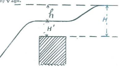
weir, the head H was always measured well upstream of the weir and then the discharge was computed by the formula,  $Q=\frac{2}{3}CL\sqrt{2g}H^{\frac{3}{2}}$  (1)
