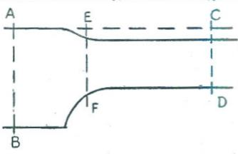
In applying the index to the broad crested weir, the Author had taken the velocity over the plane C. D. of sketch and the depth on plane A. B. Surely it would have been more correct to take the two at the same point and if this had been done, it would be obvious from consideration of any plane such as E. F. that the silt capacity must progressively increase in the curved approach and be very much higher on the crest than in the bed of the channel.
