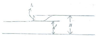
is not to be greater than 2/3 H or that drowning is not to exceed 66 per cent. This condition implies that so long as this relation is fulfilled, the discharge through the flume can be taken as a discharge through a free fall or, that discharge for it is given by the formula: Q=CLH 3/2 where:
