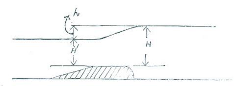
through a flume is independent of the F. Supply down-stream so long as a standing wave is formed. The moment this standing wave begins to disappear the discharge becomes dependent on "drowning" and is no longer the same as for a free fall.
