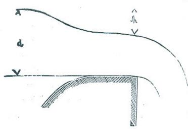
Let d be as before, and h be the drop of water surface before leaving the weir crest, under free fall conditions.
