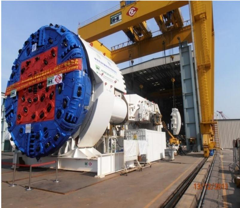
**Figure 2 : Tunnel Boring Machine (TBM) being assembled**
