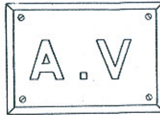
FIG: 29. INDICATING AIR VALVE.
