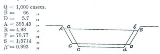
Case No. 3.—When the water surface level rises throughout. There is some silt in bed but width does not change appreciably:
