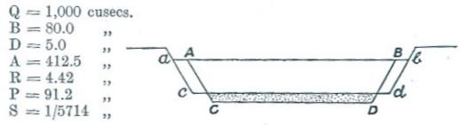
Case No. 2.—When the water surface levels and slope still remain the same, but the channel, instead of getting wider, becomes narrower and deeper, such as:
