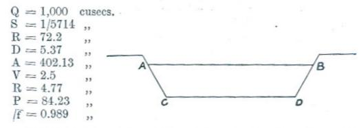
Consider the changing phases of the site in digging only. After some time the shape of the channel is changed and these changes could be represented as under:
