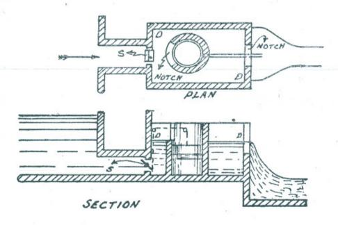
This module is similar to the one described above in use on the Henares Canal. The only difference is that the manual control of the sluice is done away with and is replaced by an automatic control. The shutter at S is controlled by a float in the intermediate chamber DD.
