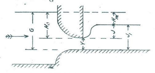
In the case of an O. S. M. it is the ratio of the height of the jump to the depression head, viz.,  $\frac{J}{H_s}$ .
