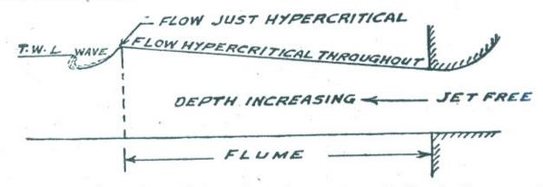
Mr. Crump has shown that the action of the baffles merely depends on the sensitive conditions (as regards the depth of flow) which are known to attend the critical state of flow. He has calculated that if the flow is hyper-critical with the total head (D) one per cent in excess of critical, the decrease in depth, relative to critical depth is:
