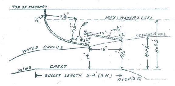
discharge. The greater the rise of the water level in the channel and the consequent increase in the velocity of discharge through the flume the greater is the reverse pressure exerted by the flow between the plates in the opposite direction. By a suitable manipulation of
