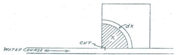
3. Theory of flow. Assume that at time t hours, after a watercourse has been cut into a field, X acres have been irrigated, i. e., water is standing over X acres with a depth of  $\delta$  inches.
