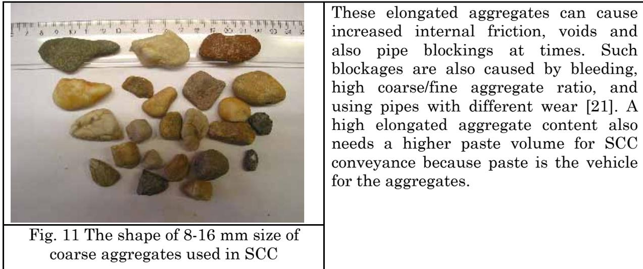
Fig 11 shows the shape of 8-16 mm size coarse aggregates used in SCC. According to above mentioned DIN standard, it was evaluated and was found a border line case with 15% elongated aggregates.
