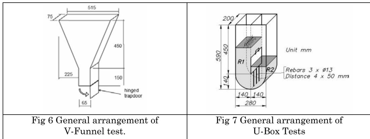
The bottom gate is opened either immediately or after 1 minute (German and Canadian practice respectively) and the time required for the concrete to flow through the opening is measured.
