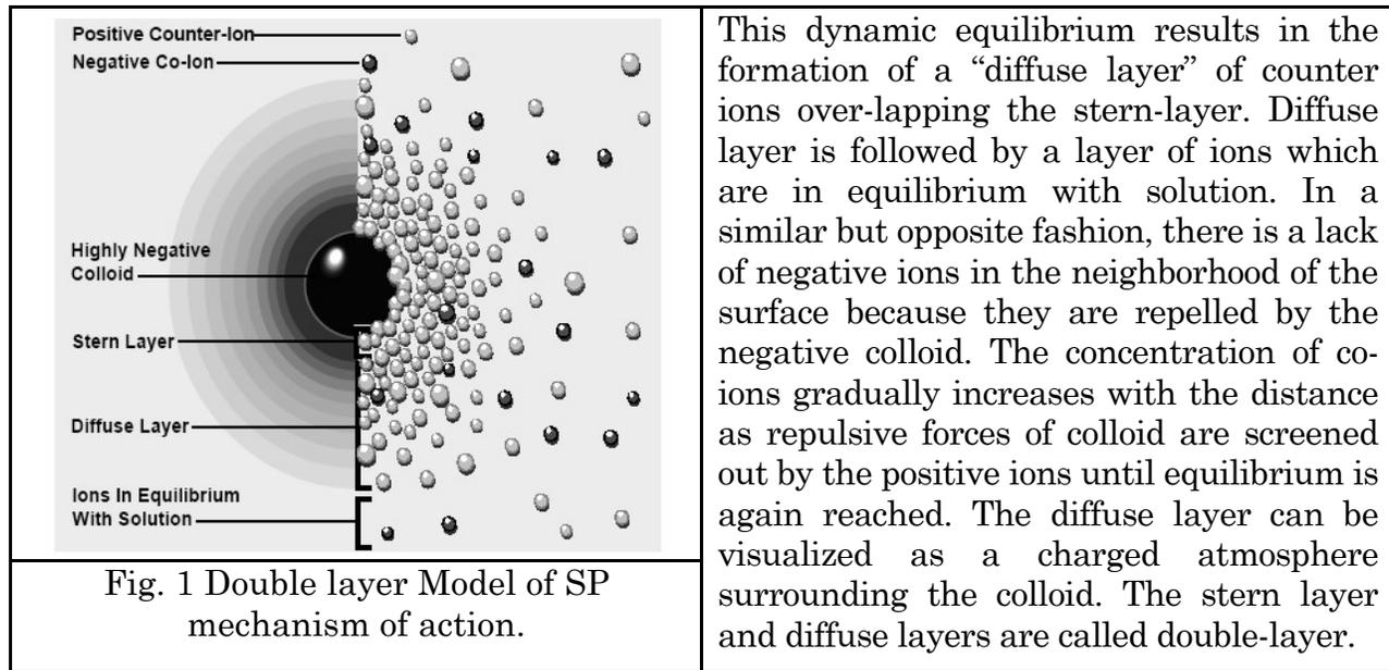
Fig. 1 Double layer Model of SP mechanism of action.
