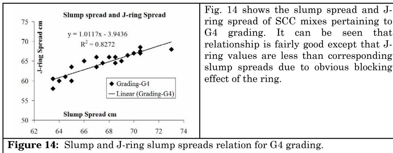
**Figure 14:** Slump and J-ring slump spreads relation for G4 grading.
