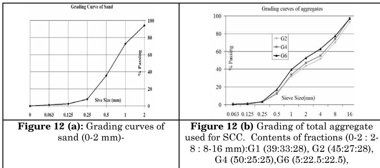
**Figure 12 (a):** Grading curves of sand (0-2 mm)-
