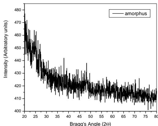
Fig 1- X-ray diffraction pattern as synthesized  $\text{TiO}_2$  nano particles.
