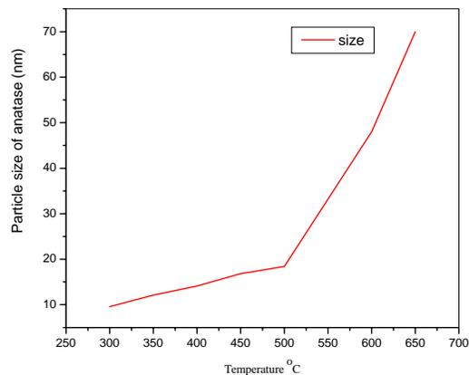
Fig 3- Variation of particles size as a function of calcination temperature.
