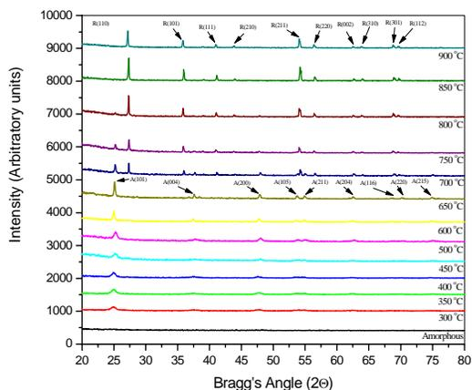
Fig 2- X-ray diffraction patterns of  $\text{TiO}_2$  annealed at various temperatures.
