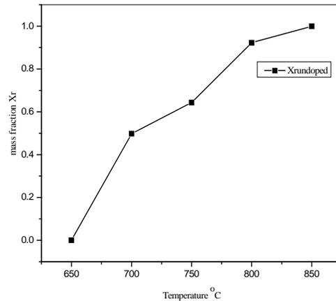
Fig 5- Effect of calcination temperature on the anatase to rutile phase transformation for TiO<sub>2</sub> nano particles.
