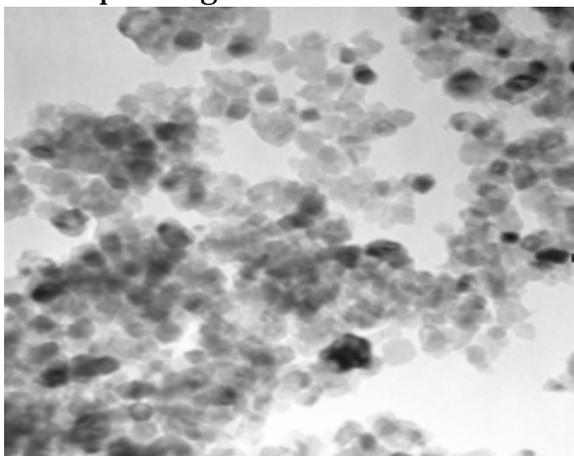
Figure 4- EM bright field image of  $\text{TiO}_2$  annealed calcined at 500°C for one hour.
