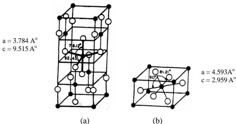
Fig. 1 Structure of anatase and Rutile TiO<sub>2</sub> (a) anatase (b) rutile
