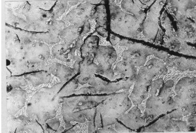
Figure 1: A microstructure of a as cast sample showing graphite flakes, pearlite and phosphide eutectic. Etchant 4% Picral. X 400
