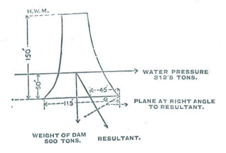
Water pressure =  $\frac{\text{w. h}^2}{2} = \frac{1}{36} \times \frac{150^2}{2} = 312.5$  tons, the weight of water being  $\frac{1}{36}$ th of a ton per cubic foot.
