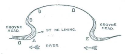
The maximum depth of water at A was fifty-five feet when only waist deep at D. D. The point 'A' gave no trouble, but the points B and C suffered severely from back water, and required constant attention during the first flood season, the river trying, as it were, to cut through the neck B C.
