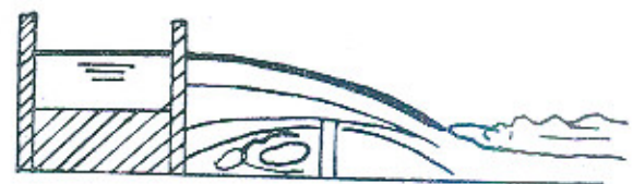
Fig. 5—Rectangular Weir without Contraction
